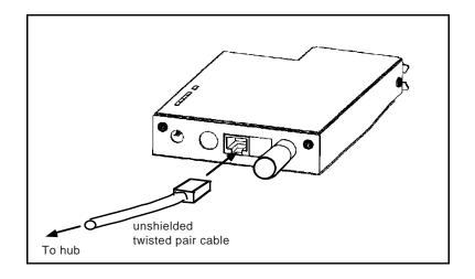
Figure 2-4 Connecting the Print Server to a 10baseT UTP network
